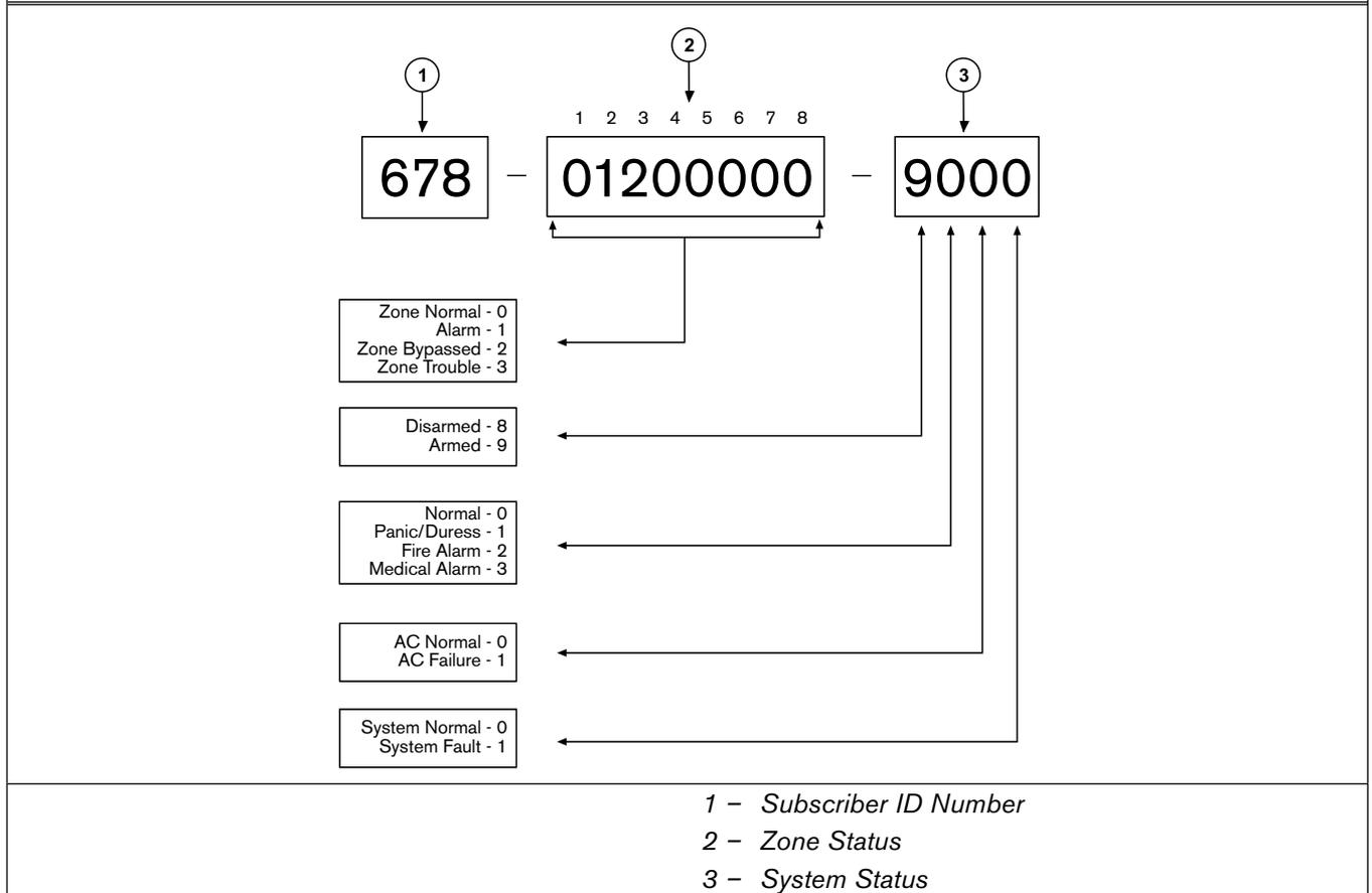
Figure 8 shows the transmission came from the control panel with an ID number of 678 and that zone 2 is in alarm. The figure also displays that zone 3 was manually isolated and the system armed.
